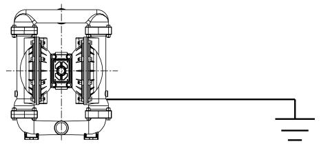
This Ground Strap (Item 34) is shipped with the eyelet end fastened to the pump hardware.
