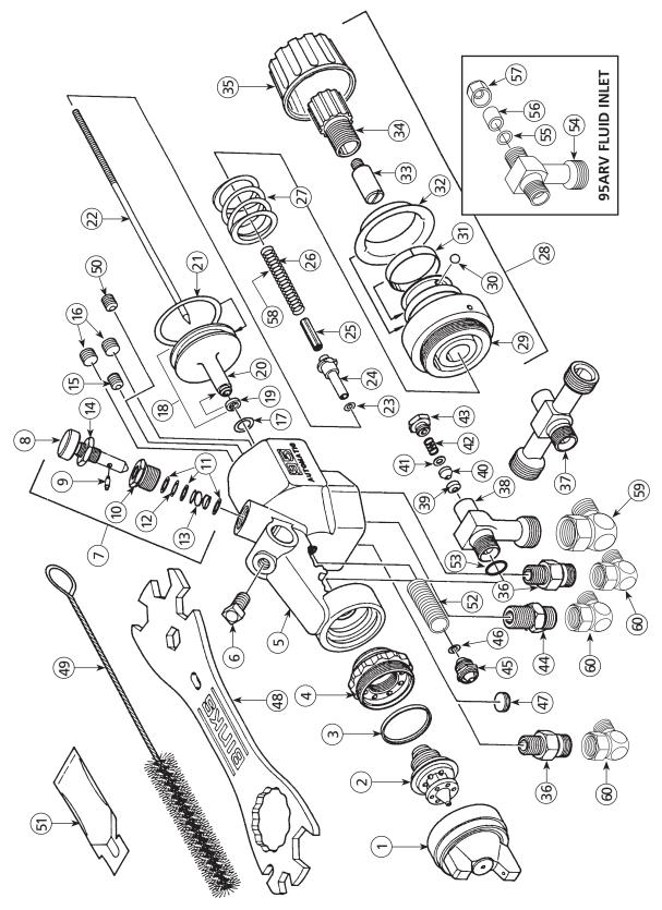
▲Items (36) and (50) are for installations requiring separate fan and atomizing air control. Items are packaged loose. (See pg. 5)
