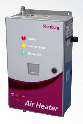
In automated finishing applications, the expansion of pressurized air results in condensation. The Ransburg Air Heater is designed to reduce or eliminate condensation that may form in or on TurboDisks, Air Turbines, Fluidized Powder Beds or other pressurized applicators under certain operating conditions.
