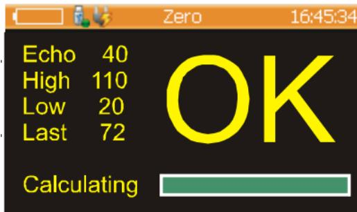
**Note:** In the unlikely event of a zeroing failure an error code will be displayed. Check the zero reference block for contamination or damage and retry. In the case of multiple failures please contact your nearest Elcometer representative.
