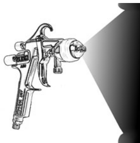
HVLP Low Pressure Spray Gun Overspray
