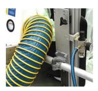
Feed the edge of the masking sheet between the hood and the masking band all the way round the hood to create a good seal between the panel and the hood.
