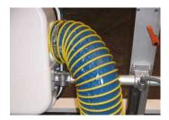
Connect the hood hose to the extraction tower hose using the quick release connections. Check the condition of the hood filter and that it is secured in the correct position.
