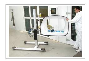
Walk around the base, hood and mast assembly until it locates in its new position.
