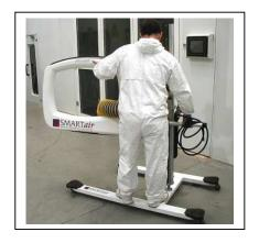
Ensure there is enough space around the stand to allow easy movement. Stand on base and lift mast and hood assembly approx 25mm upwards and slightly turn to mast.
