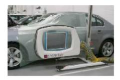
Position the hood over the centre of the area to be painted. The back edge of the hood (with rubber protection) should be positioned to within 50mm (2") of the panel to be painted. Use the horizontal and vertical adjustment handles to loosen and fix the hood position.
