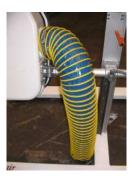
Check the condition of the extraction hose. There should be no perforations, which will allow air to enter the hose other than through the hood connection. Report any damage immediately.
