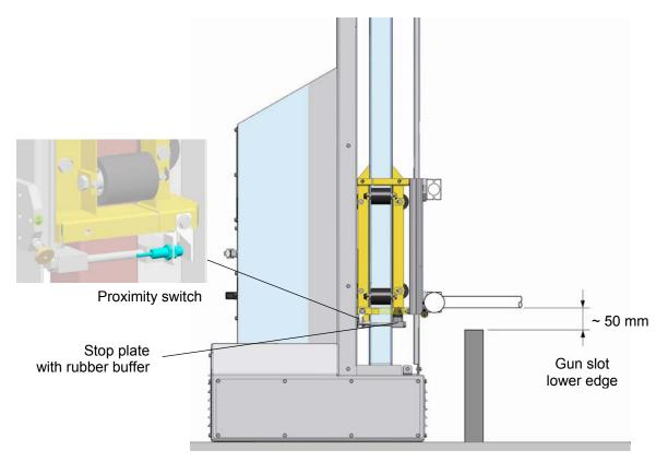
ZA06 reciprocator - reference point and mechanical stops
