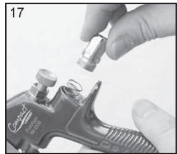
17. Replace Valve Spring and screw in Housing (10).
