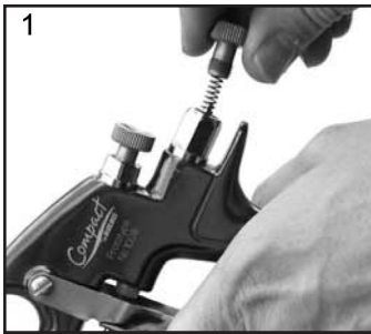
1. Remove Adjusting Knob (7), Spring (8), and Needle (9).
