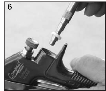
6. Remove Valve Seat.
