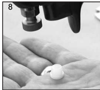
8. Turn the Gun upside down and let the Seal fall out.
