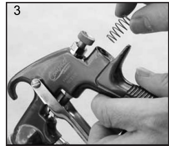
3. Remove Housing (10) and Air Valve Spring.
