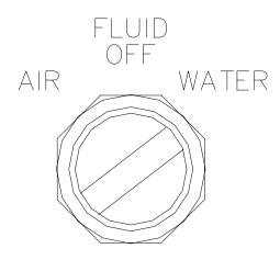
Figure 18: Fluid Selection Switch for Water Tests
