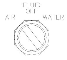
Figure 10: Fluid Selection Switch
