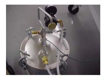
Figure 3: Fluid and Air Line Connections
