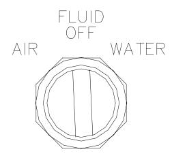
Figure 19: Fluid Selector Switch "Off" Position
