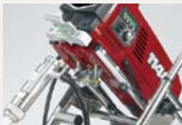
Pull handle under body down. Slide out fluid section
