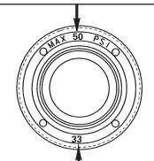
Air cap number located on face of cap cap number must correspond with baffle number to assure 10 PSI cap pressure.
