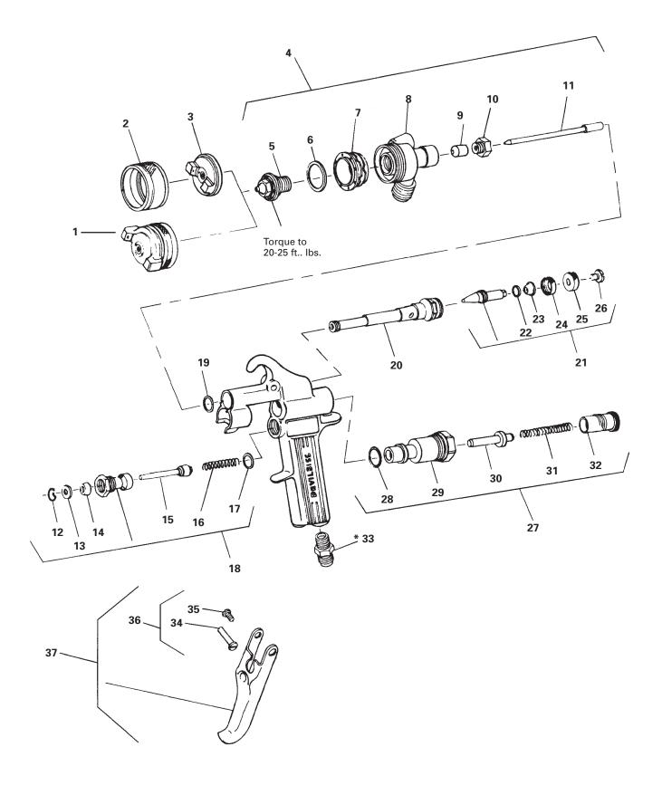
\*Apply thread sealant (i.e. Loctite 242, blue or equal) on threads.
