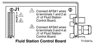
Fig. 18: Servicing Air Flow Switch
