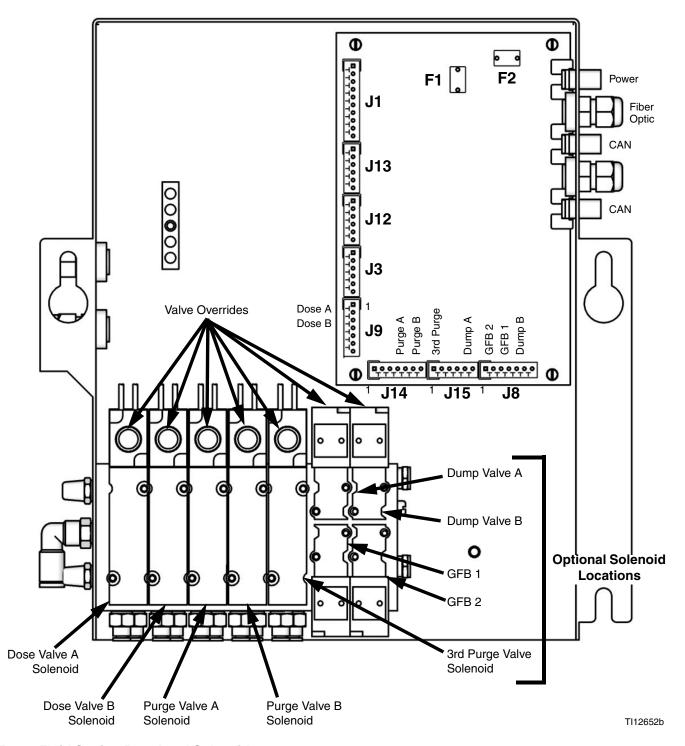
Fig. 4: Fluid Station Board and Solenoids
