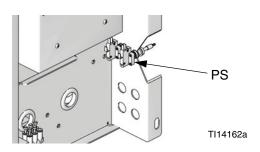
Fig. 19: Servicing GFB Pressure Switch
