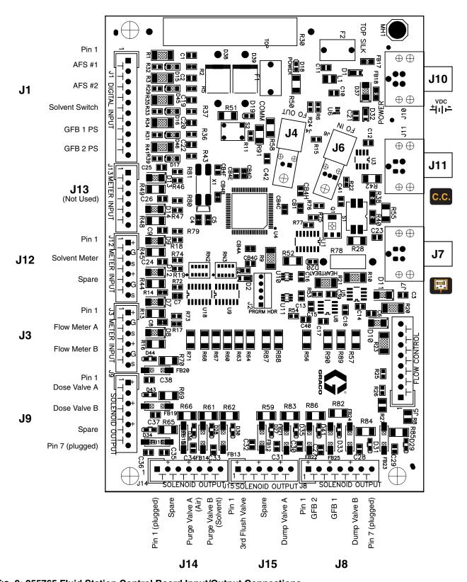
Fig. 9: 255765 Fluid Station Control Board Input/Output Connections
