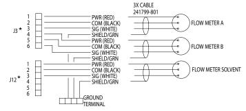
\*Connectors on Fluid Station Control Board
