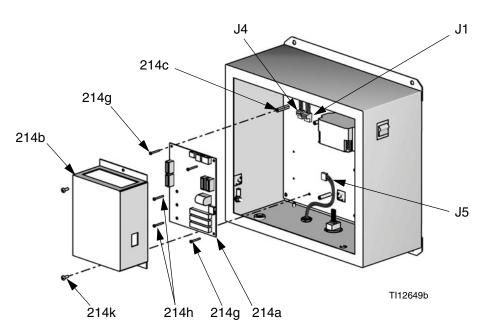
Fig. 15: Replacing Barrier Board
