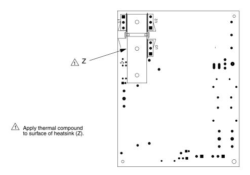
Back of Barrier Board, showing Heatsink (Z)
