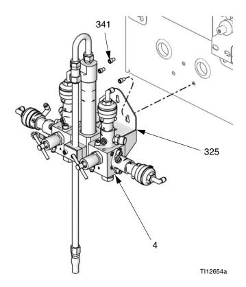
Fig. 25: Fluid Manifold
