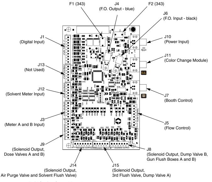
Fig. 21: 255765 Fluid Station Control Board
