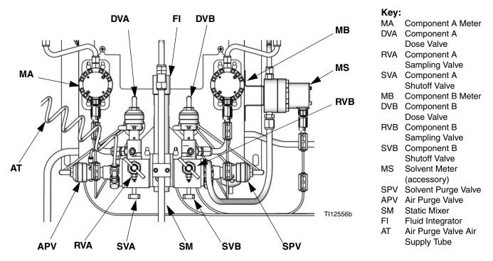
Fig. 3. Wall Mount Fluid Station
