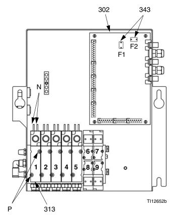
Fig. 22: Replacing Solenoids and Fuse
