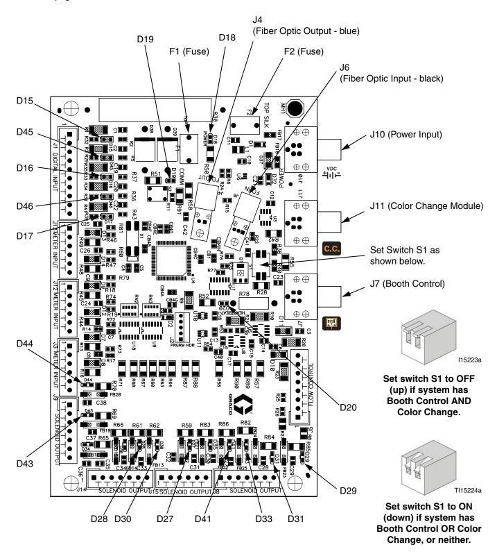
Fig. 8: 255765 Fluid Station Control Board Indicators
