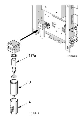
Fig. 17: Replacing Air Filter Element
